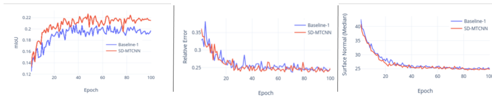
Figure 1: Performance graph between SD-MTCNN (Eq. 5 main paper) and SD-Vanilla Segnet (Baseline-1 main paper) for three tasks on the NYUv2 dataset. From left to right: mIoU (semantic segmentation), relative error (depth estimation), and median error (surface normal).
